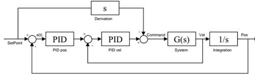
Fig.5: Scheme of controller
