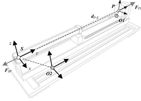
Fig.3: *Main references for the pneumatic "constraint object"*
