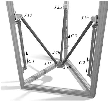
Fig.6: Three-dimensional multibody simulation of TORX robot
