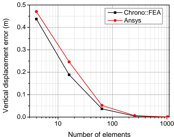
Figure 2: Convergence analysis of static deflection under the action of a load
