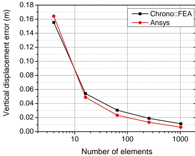
Figure 3: Convergence analysis of static deflection under the action of a load for Mooney-Rivlin material
