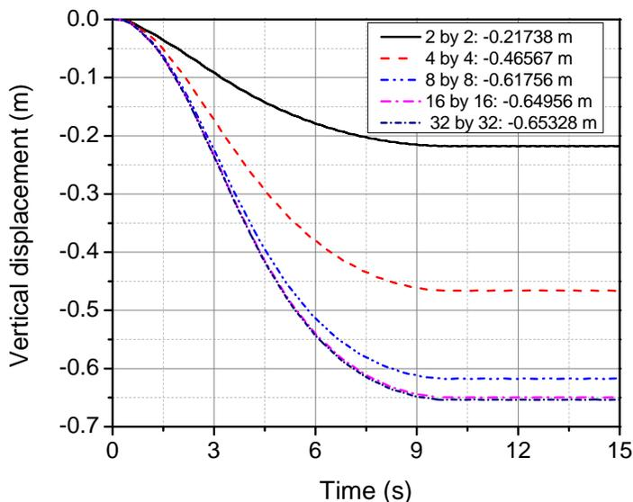
Figure 1: Dynamic evolution of a bricked plate tip under a gradually applied load of 50N
