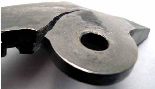
Fig.3: Structural failure of old pliers
