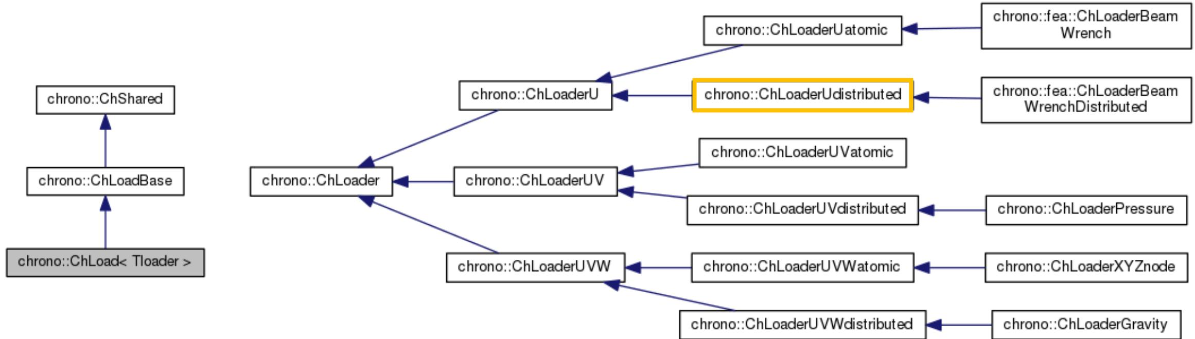
ChLoad inheritance tree: allows the user to apply loads to an FEA mesh in a convenient way
